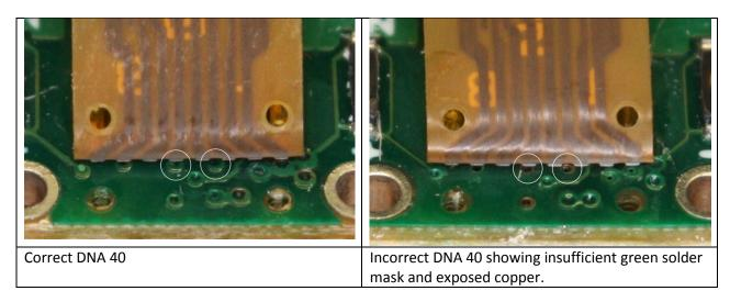
The corrective action for boards with this problem is to apply a small bead of electronics-grade silicone or epoxy into the joint between the screen cable and the board as shown below. This will insulate the PCB cable from the board in these two spots.
