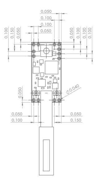
The mounting holes for the DNA 30D are .100" pitch and .040" diameter. It can be wired in directly using soldered connections, or socketed with .1" hardware.
