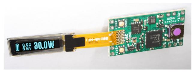
The DNA 30D is a power regulated digital switch-mode DC-DC converter for personal vaporizers. It features a small OLED display, analog or digital user controls, onboard buttons and synchronous rectification for maximum battery life and minimal heat generation.
