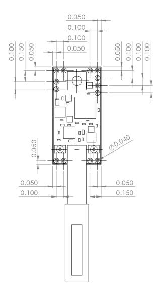
The mounting holes for the DNA 20D are .100" pitch and .040" diameter. It can be wired in directly using soldered connections, or socketed with standard .1" hardware.
