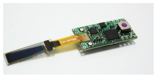
The DNA 20D is a power regulated digital switch-mode DC-DC converter for personal vaporizers. It features a small OLED display, analog or digital user controls, onboard buttons and synchronous rectification for maximum battery life and minimal heat generation.
