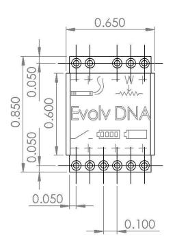
The mounting holes for the DNA 12 are .100" pitch. It can be wired in directly using soldered connections, or socketed with standard .1" hardware.
